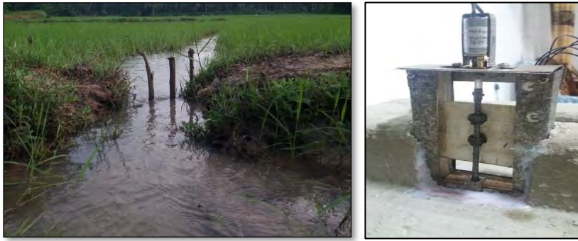
Figure 1: Traditional WAKKADA & Prototype sluice gate mechanism
