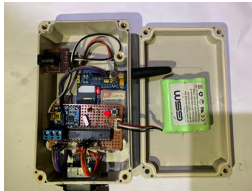
Figure 3(c): Inside of the Electric Fence Fault Finding System
