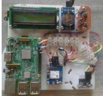
Figure 2: Device to collect Vehicle Data
