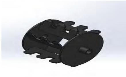
Figure 4: Plough Type Weeding Mechanism
